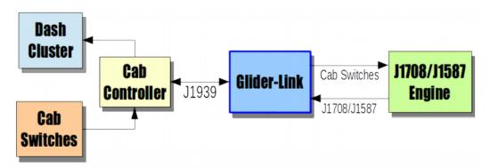
Illustration 1: Vehicle & Glider-Link Block Diagram
