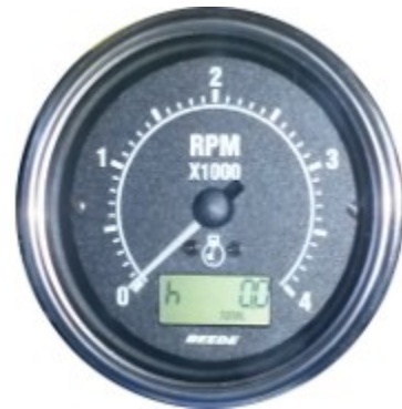
Proper needle location when ignition is on. After corrective measures.
