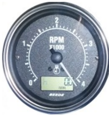
Appearance at stuck position after emergency shut down & ignition is turned back on.
