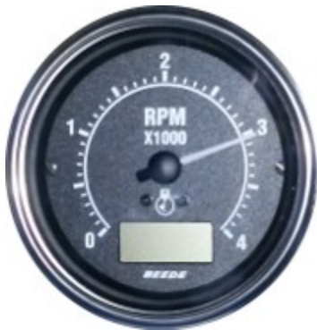
Typical needle location after emergency shut down.
